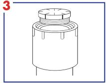
Hand tighten the Sewer Popper in place of the plug.
